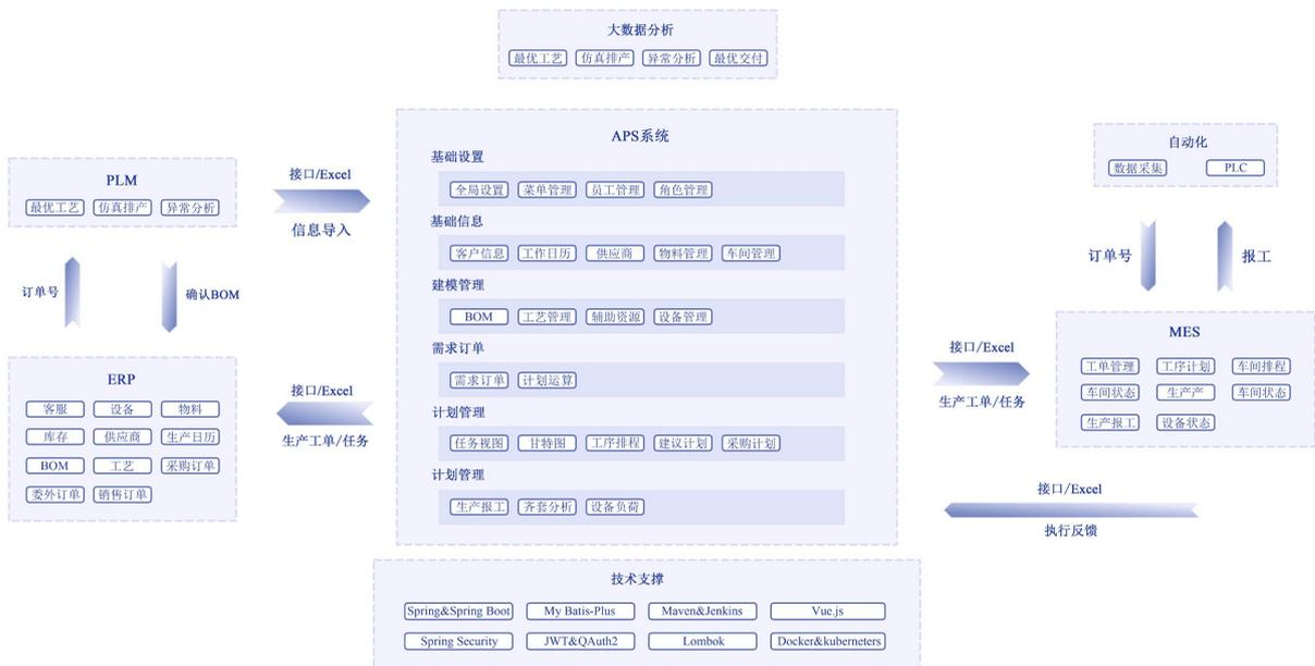
Figure 2. APS system module diagram
