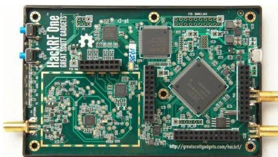
Figure 1. HackRF One device
