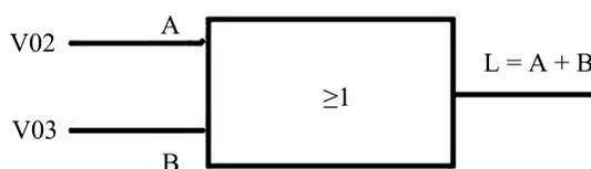
Figure 12. OR gate circuit
