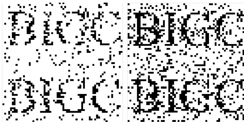
Figure 17. Video frames after the video is passed through the motion blur filter and the extracted watermark 图 17. 视频经过运动模糊滤镜后的视频帧和提取出的水印
