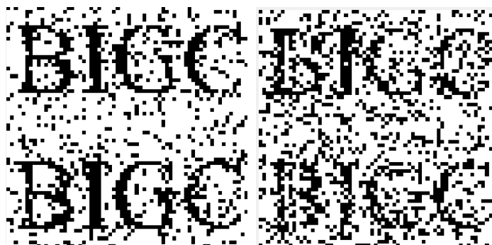
Figure 7. Watermark of the two videos after mean filtering and decryption of the carrier image 图 7. 两个视频遭受均值滤波后载体图像解密后的水印
