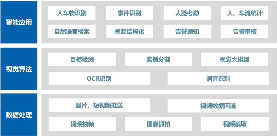
Figure 7. Function architecture of the video intelligent analysis module 图 7. 视频智能分析模块功能架构
