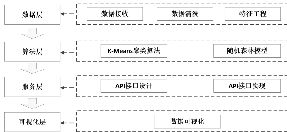
Figure 1. System overall architecture diagram 图 1. 系统整体架构图
