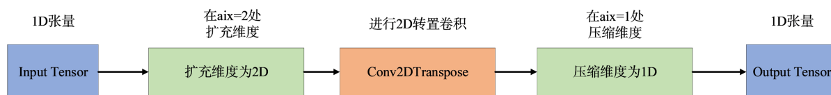
Figure 5. 1D Transposed convolution module
