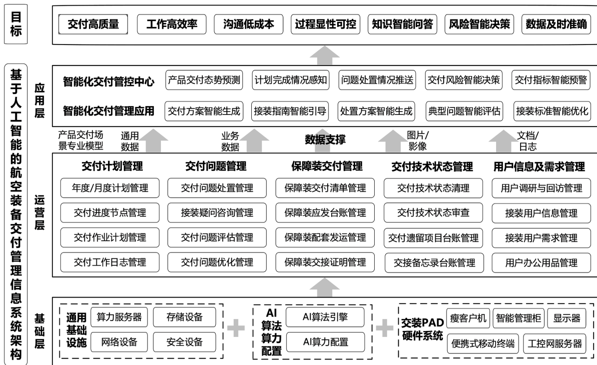
Figure 3. Artificial intelligence-based information system architecture for aircraft product delivery management
