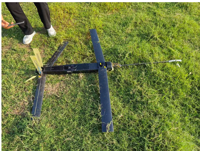
Figure 11. Installation and layout of the magnetometer on the small fixed-wing UAV 图 11. 小型固定翼无人机磁探仪安装布置图
