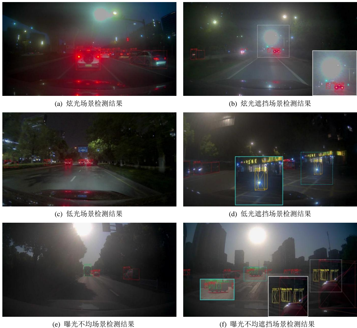
Figure 4. BEVFusion target detection results in complex lighting scenarios
