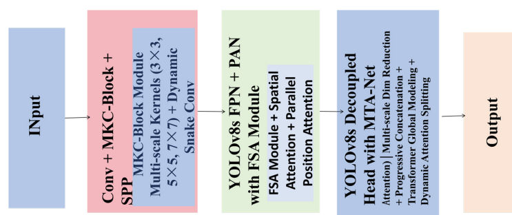
Figure 1. YOLOv8s-MSFDS model architecture diagram
