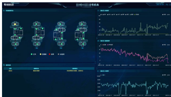
Figure 6. Health assessment system sub-health warning diagram for locomotive No. 16 图 6. 某机车 16 位健康评估系统提示图(亚健康)
