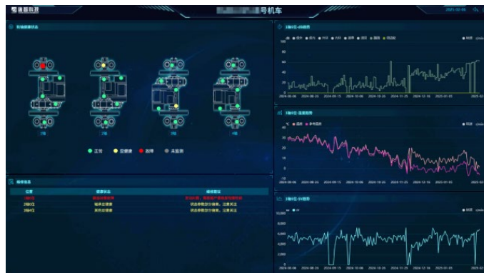
Figure 7. Health assessment system minor fault warning diagram for locomotive No. 16 图 7. 某机车 16 位健康评估系统提示图(轻微故障)
