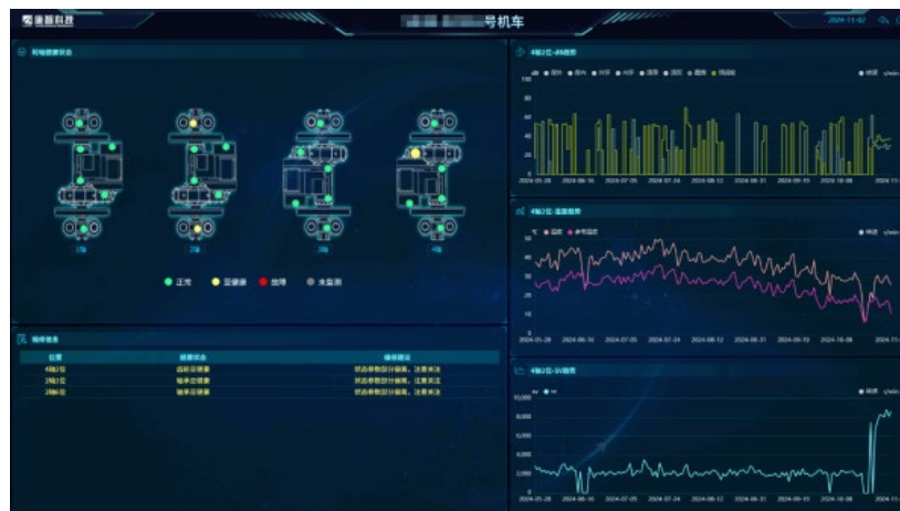
Figure 4. Health assessment system warning diagram for locomotive No. 42, November 2024
