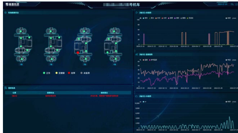
Figure 3. Minor fault warning diagram of health assessment system for locomotive No. 35
