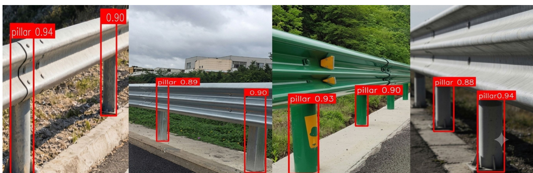
Figure 8. Qualitative detection results of the baseline YOLOv5s algorithm 图 8. YOLOv5s 算法检测结果
