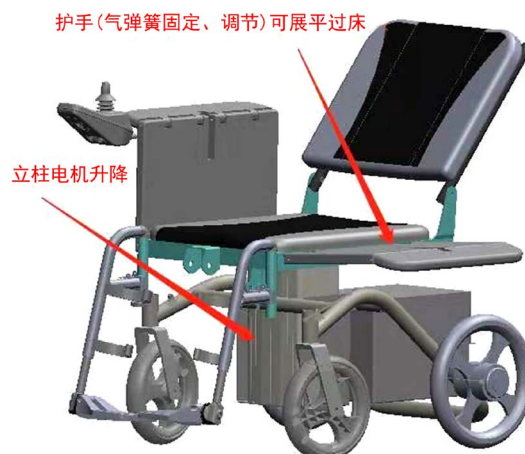
Figure 1. Basic design of wheelchair for hemiplegic patients
