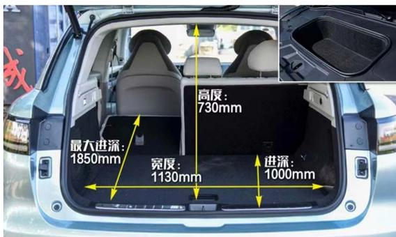
Figure 3. Leapmotor C11 trunk data
