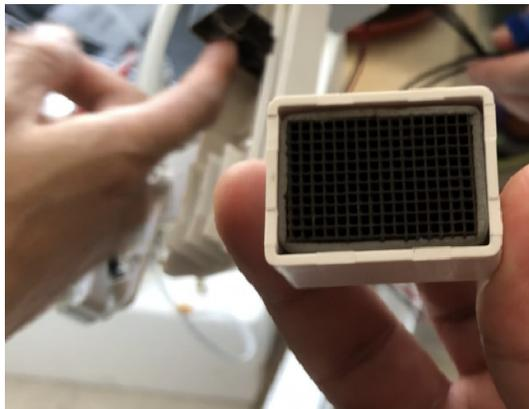
**Figure 2.** Activated carbon deodorization in smart toilets
