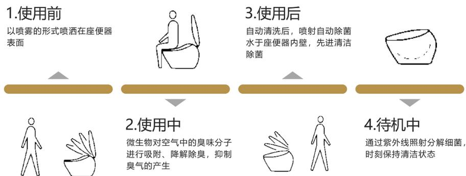
**Figure 5.** Smart toilet deodorization process
