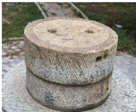
Figure 1. Upper and lower stone grinding discs
