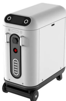
Figure 4. E-BOX charging robot
