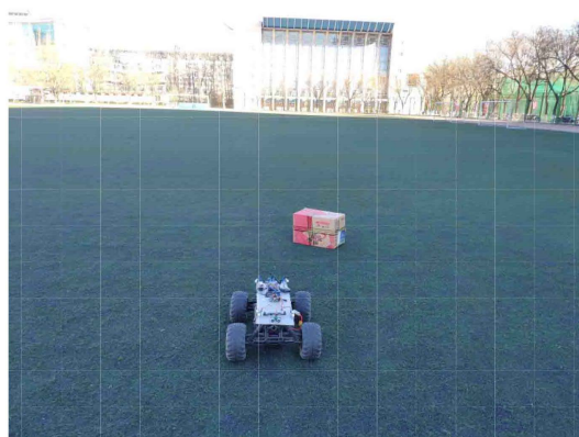
Figure 19. U2, U3 ultrasonic detection of obstacles
