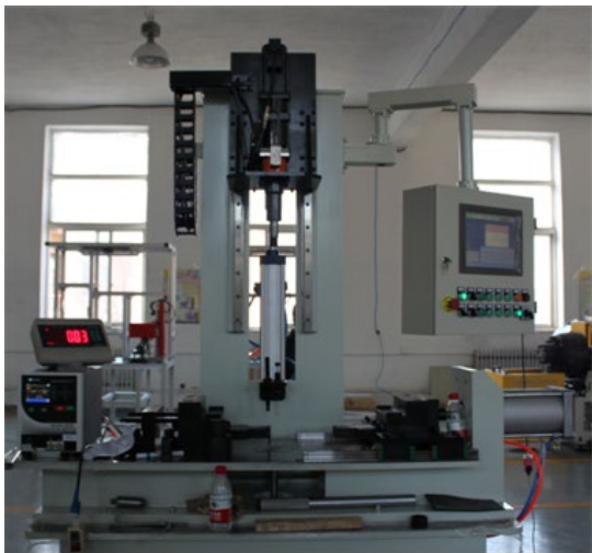
Figure 9. Prototype of solid rocket automated assembly equipment 图 9. 固体小火箭自动化装配设备样机
