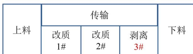
Figure 1. Fully automatic laser lift-off line sketch
