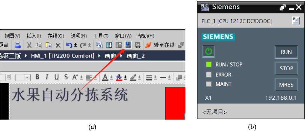
Figure 10. Platform construction and simulation startup interface; (a) Start the PLC simulation; (b) PLC module startup 图 10. 平台搭建与仿真启动界面。(a) 启动 PLC 仿真；(b) PLC 模块启动
