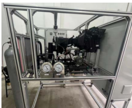
Figure 1. \text{CO}_2 heat pump air conditioning system experimental bench 图 1. \text{CO}_2 热泵空调系统实验台架
