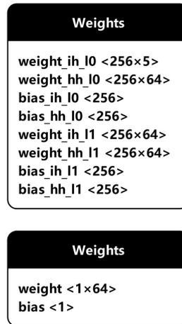
Figure 2. LSTM model structure diagram
