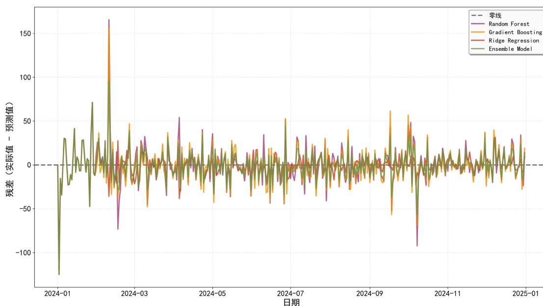
Figure 4. Comparison of residuals for random forest, gradient boosting, ridge regression, and ensemble models
