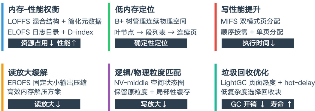
Figure 4. File system optimization techniques in embedded operating systems 图 4. 嵌入式操作系统中的文件系统优化技术
