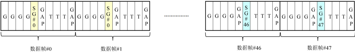
Figure 3. Schematic diagram of the NearLink ultra-short frame structure 图 3. 星闪超短帧结构示意图
