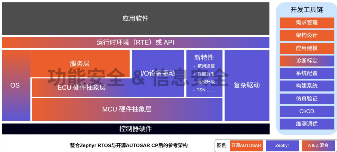
Figure 8. The reference software platform combined Zephyr and AUTOSAR CP
