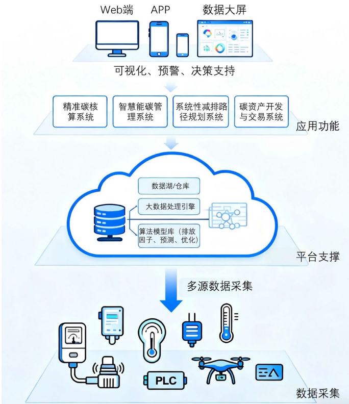
Figure 1. Overall technical architecture of carbon management digital platform for marine ranching enterprises 图 1. 海洋牧场企业碳管理数字化平台整体技术架构图
