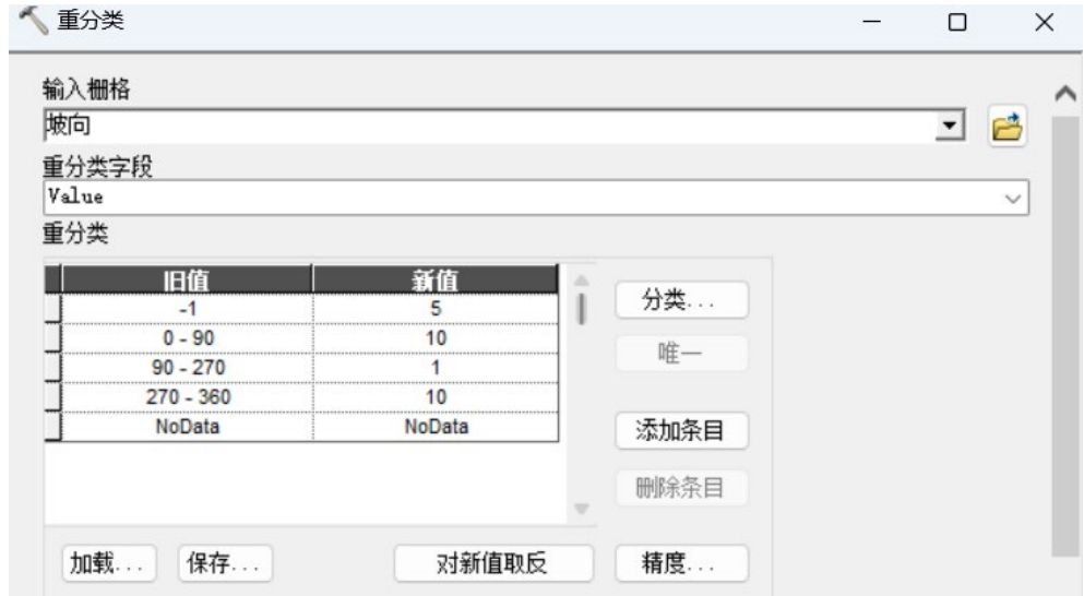
Figure 4. Slope reclassification comparison table 图 4. 坡向重分类对照表
