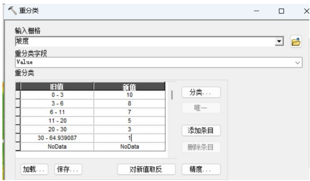
Figure 3. Critical value for slope reclassification 图 3. 坡度重分类临界值
