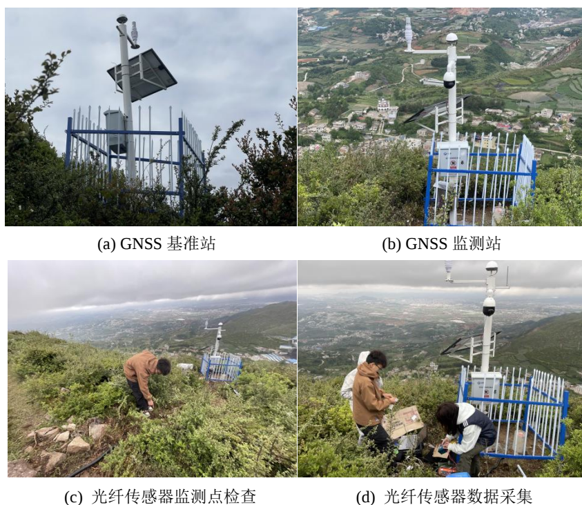
Figure 2. GNSS and distributed optical fiber sensing acquisition system 图 2. GNSS 和分布式光纤技术采集系统
