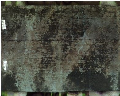
Figure 9. Argillaceous coarse-grained sandstone with wavy lamination 图 9. 含泥波状层理粗砂岩
