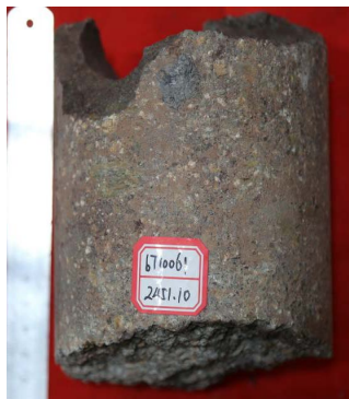
Figure 6. Reddish-brown clast-supported fine-grained conglomerate with randomly arranged grains 图 6. 红褐色杂乱排列颗粒支撑细砾岩
