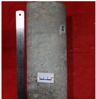
Figure 8. Cross-bedded pebbly coarse-grained sandstone with wavy lamination 图 8. 波状层理含砾粗砂岩
