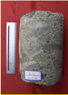
Gray Clast-Supported Coarse-Grained Conglomerate Facies with Imbricated Arrangement 灰色叠瓦排列颗粒支撑粗砾岩相
