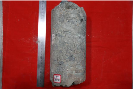
Figure 1. Clast-supported conglomerate with randomly arranged grains 图 1. 杂乱排列颗粒支撑粗砾岩
