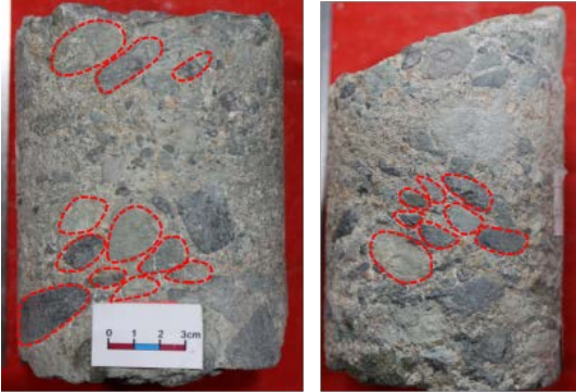
Figure 3. Clast-supported medium-grained conglomerate with imbricated grains 图 3. 叠瓦排列颗粒支撑中砾岩
