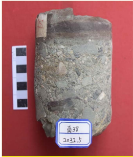
Gray Clast-Supported Fine-to-Medium-Grained Conglomerate with Imbricated Arrangement 灰色叠瓦排列颗粒支撑细-中砾岩
