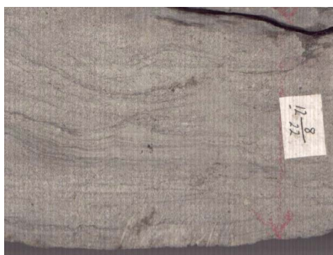
Figure 13. Siltstone with horizontal lamination
