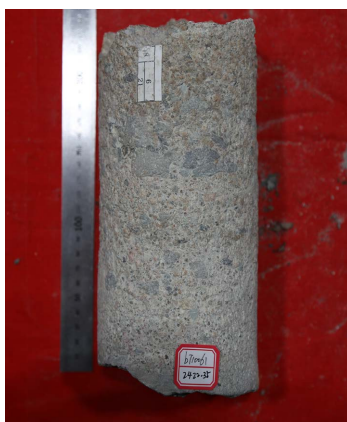
Figure 5. Clast-supported fine-grained conglomerate with imbricated grains 图 5. 叠瓦排列颗粒支撑细砾岩
