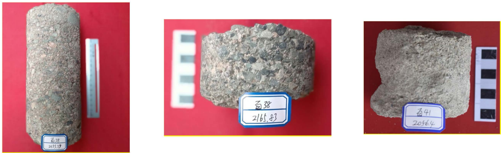
Gray Clast-Supported Fine-Grained Conglomerate Facies with Chaotic Arrangement 灰色混杂排列颗粒支撑细砾岩相 Gray Clast-Supported Fine-Grained Conglomerate Facies with Parallel Arrangement 灰色平行排列颗粒支撑细砾岩相 Gray Massive-Bedded Coarse-Grained Sandstone Facies 灰色块状层理粗砂岩相
