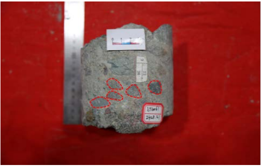
Figure 2. Clast-supported conglomerate with imbricated grains 图 2. 叠瓦排列颗粒支撑粗砾岩
