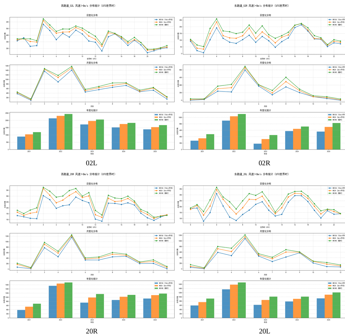
Figure 8. Statistics for wind speed exceeding 8 m/s at runway thresholds (Top to bottom: diurnal, annual, interannual variation; Blue: 10-min mean wind, Orange: 2-min mean wind, Green: instantaneous wind)
