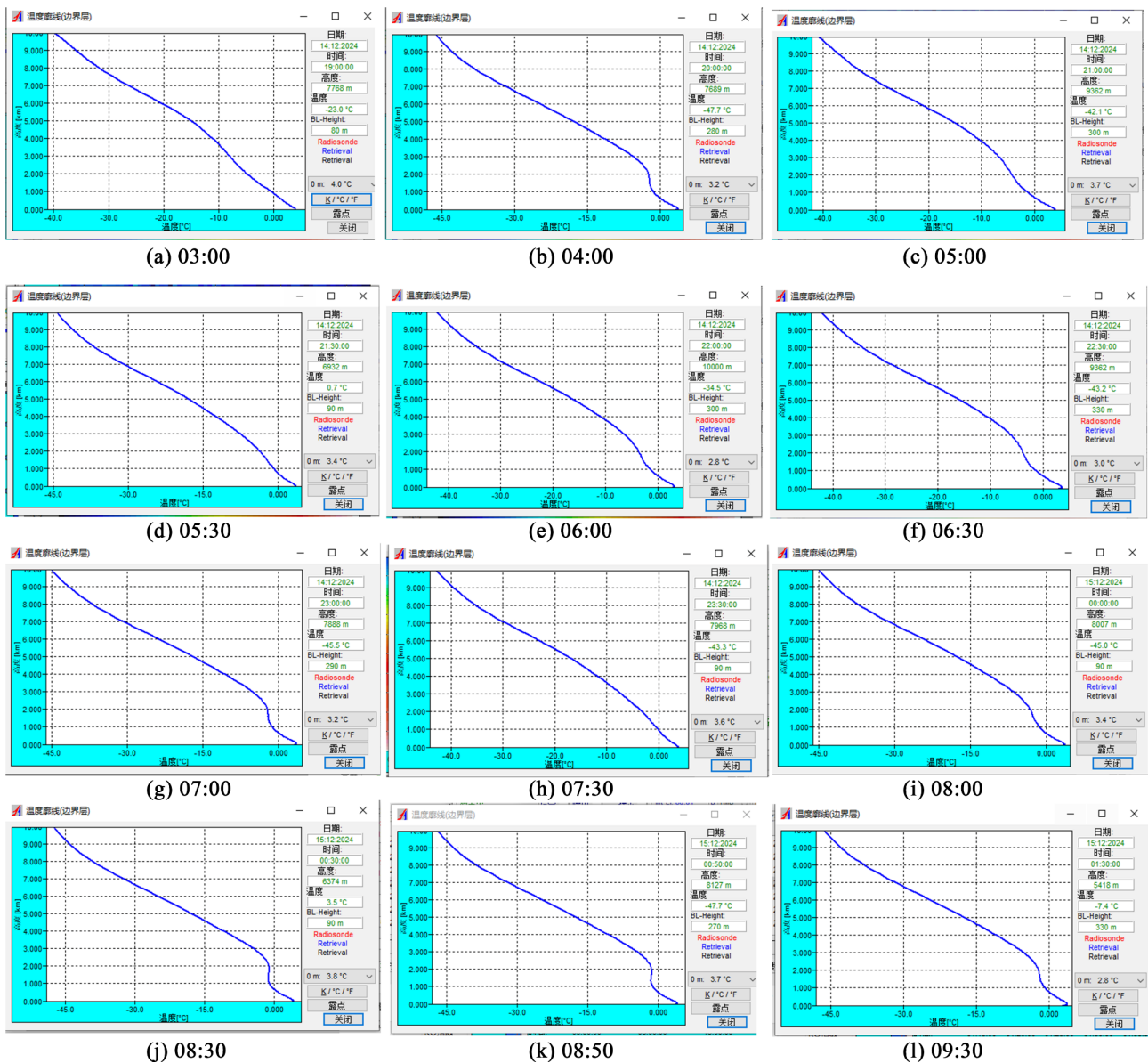
Figure 9. Temperature profile map of airport microwave radiometer from 03:00 to 09:30 in the early morning of the 15 th (Beijing time) 图 9. 15 日凌晨(03:00~09:30 (北京时))机场微波辐射计温度廓线图
