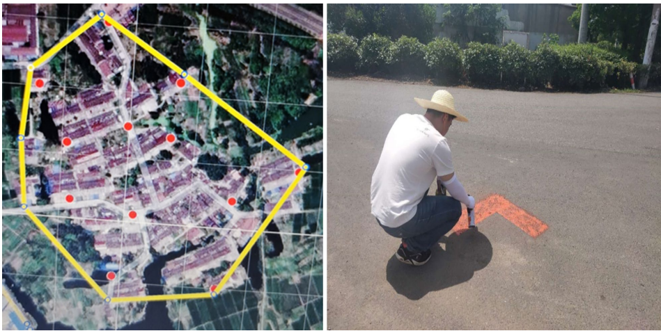
Figure 2. Layout of image control points 图 2. 像控点布设
