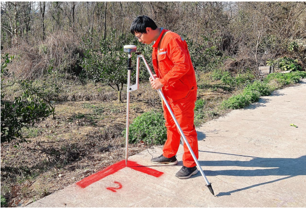
Figure 3. Image control point measurement 图 3. 像控点测量
