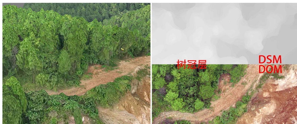
Figure 6. Schematic diagram of the 3D model and DSM model partial of aerial photogrammetry 图6. 航空摄影测量三维模型及DSM模型局部示意图
