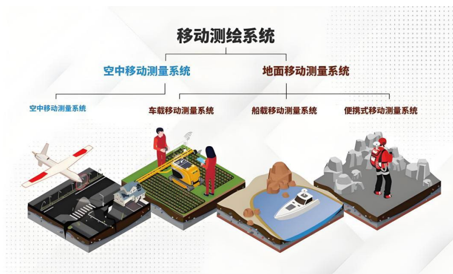
Figure 2. Classification diagram of mobile surveying and mapping systems
