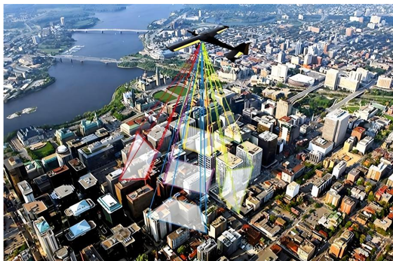
Figure 3. Schematic diagram of data collection by oblique photography technology 图 3. 倾斜摄影技术采集数据示意图
