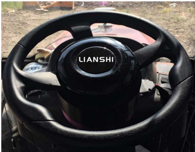
**Figure 12.** GNSS steering wheel autopilot system
