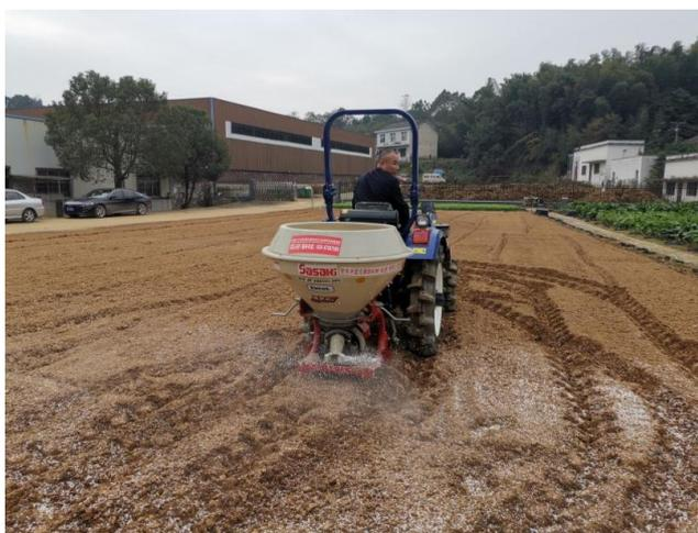
**Figure 5.** Pellet fertilizer spreader
