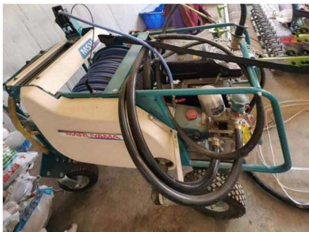
Figure 9. Self-propelled multifunctional power sprayer
