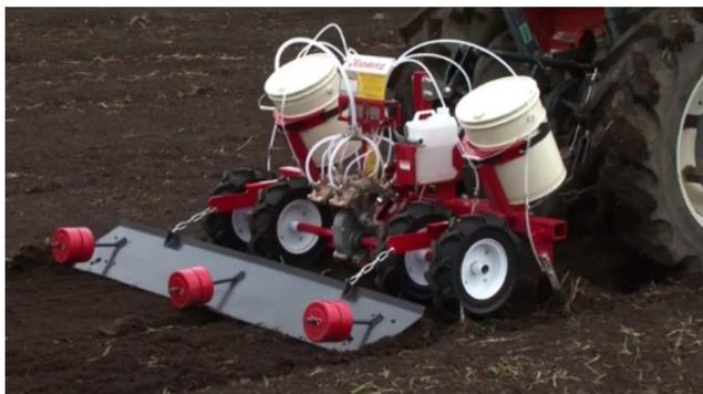
**Figure 3.** Soil disinfection machine
