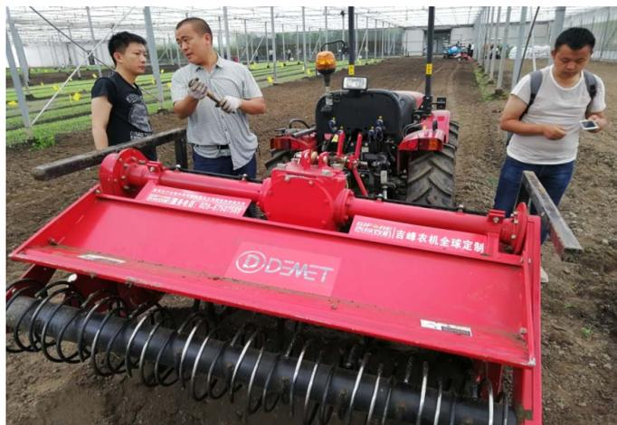
Figure 1. Soil deep loosening rotary tiller
