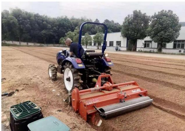
Figure 6. Ridging ditch rotary cultivation
