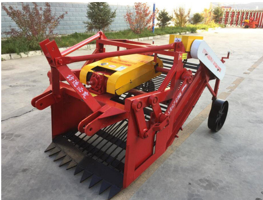
Figure 1. Vibrating screen type medicine and soil separator 图1. 振动筛式药土分离机
