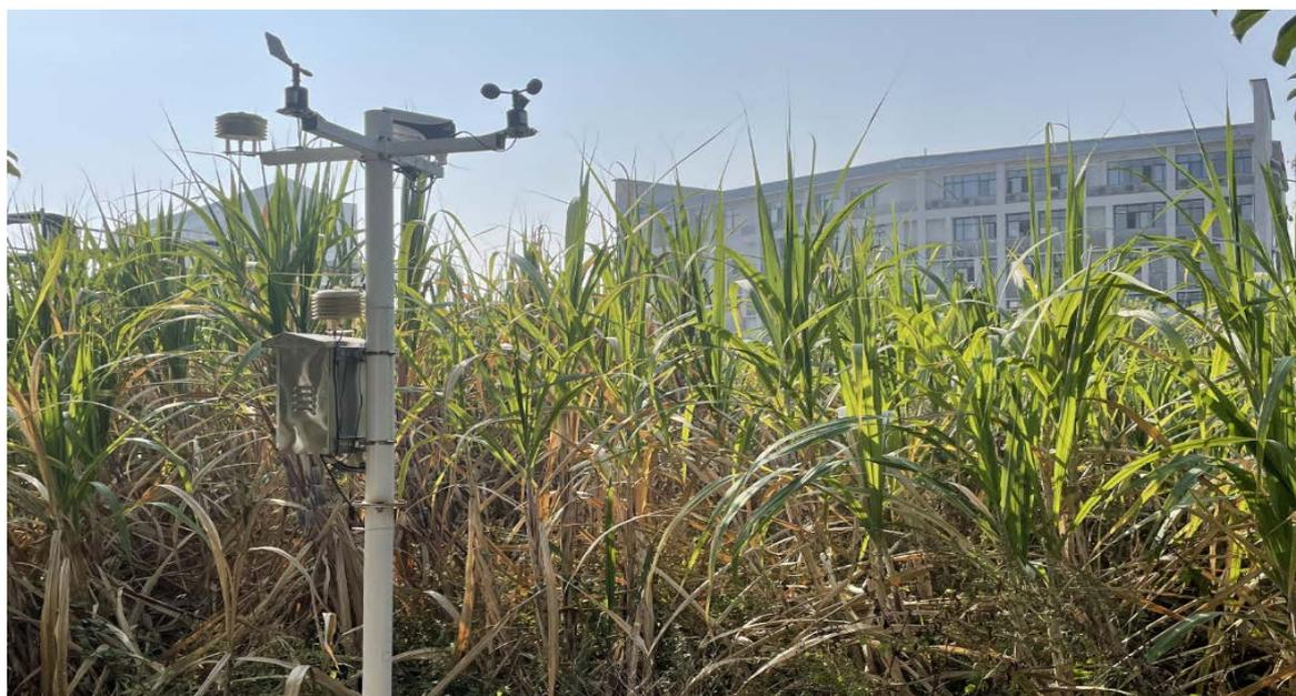
**Figure 3.** Integrated weather sensing equipment for sugarcane fields
