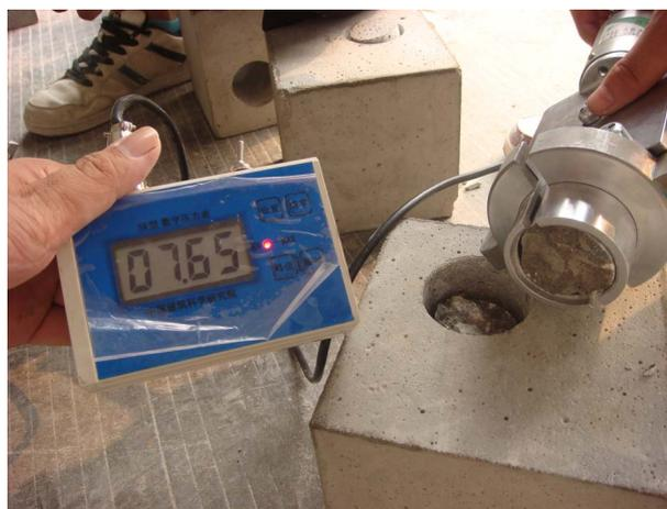
Figure 5. *In-situ* single-shearing apparatus of the shear test process
