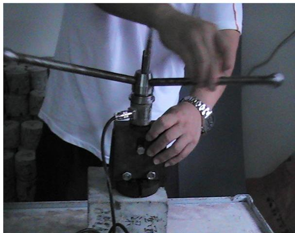
Figure 4. *In-situ* single-shearing apparatus of the shear test process
