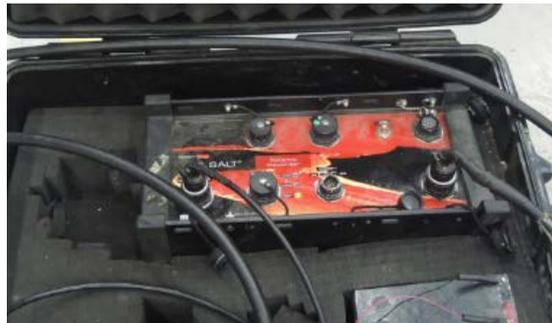
Figure 2. EpiSensor acceleration tester
