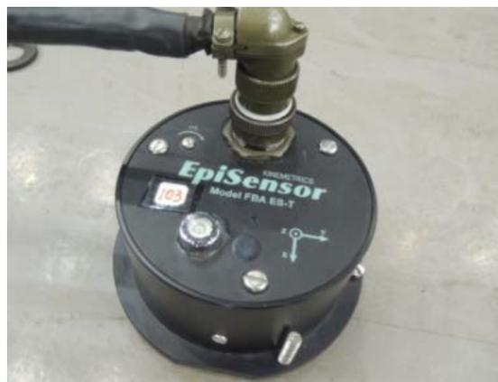
Figure 3. EpiSensor acceleration sensor
