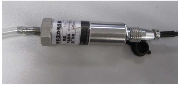
Figure 4. High precision digital pressure sensor
