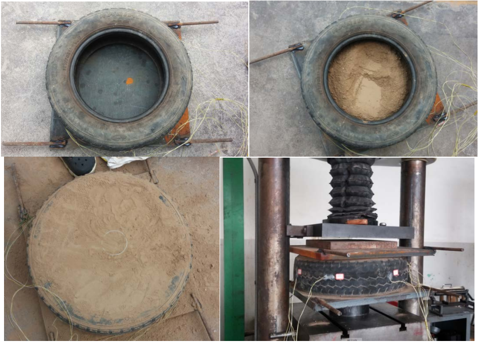
Figure 1. The filling process of tire-soil composite 图 1. 轮胎 - 土复合体填筑过程
