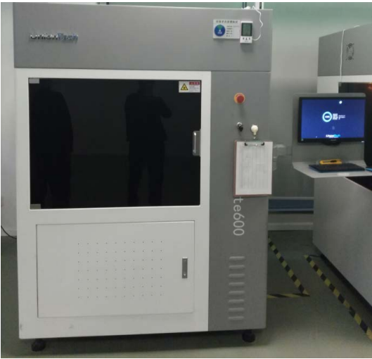
Figure 5. 3D printer based on stereo lithography apparatus 图 5. 立体光固化 3D 打印设备
