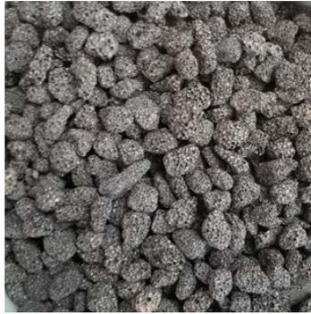
Figure 1. Foam ceramic light aggregate
