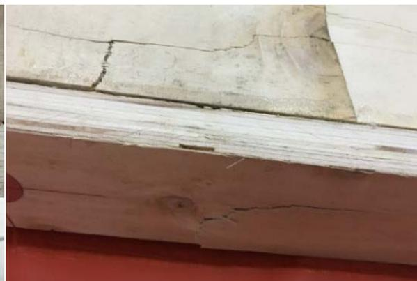
(b) 箱型梁腹板、翼缘受拉破坏
