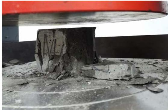
**Figure 3.** The shape of the compressive specimen after failure
