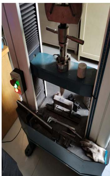
**Figure 2.** 100 t electronic universal testing machine (flexural test)
