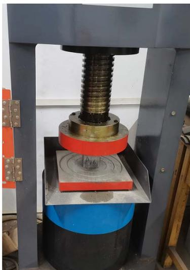
**Figure 1.** 200 t electronic universal testing machine (compression test)
