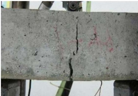
**Figure 4.** Form after failure of flexural specimen
