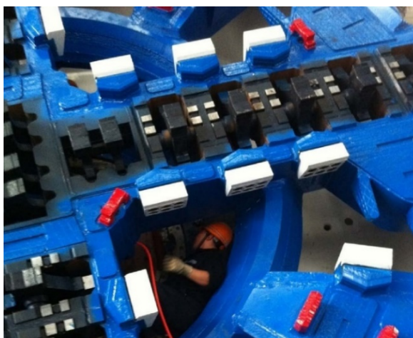
Figure 11. Shield cutter head diagram
