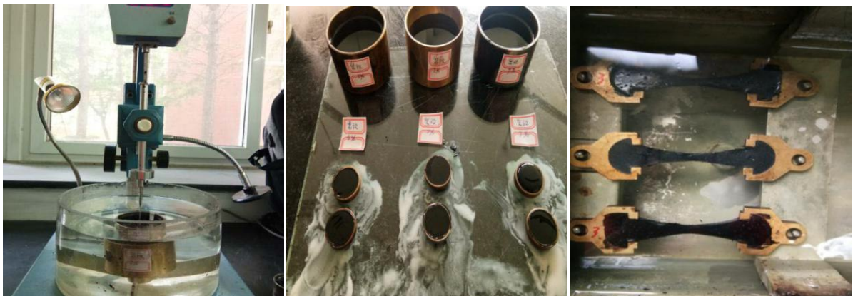
Figure 4. Routine performance test of various asphalts after TFOT 图 4. TFOT 后各种沥青常规性能试验
